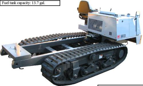
Performance Slope climbing ability: 30 deg. unloaded Ground pressure (empty): 2.28 psi Ground pressure (loaded): 4.55 psi Min. turn radius: 5.9'
